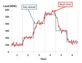
Figure 1: Day-ahead generation scheduling vs. real-time load-balancing needs
