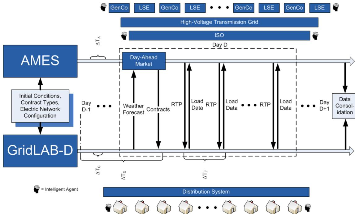
Figure 4: Seaming AMES with GridLAB-D: Co-simulation software data exchange
