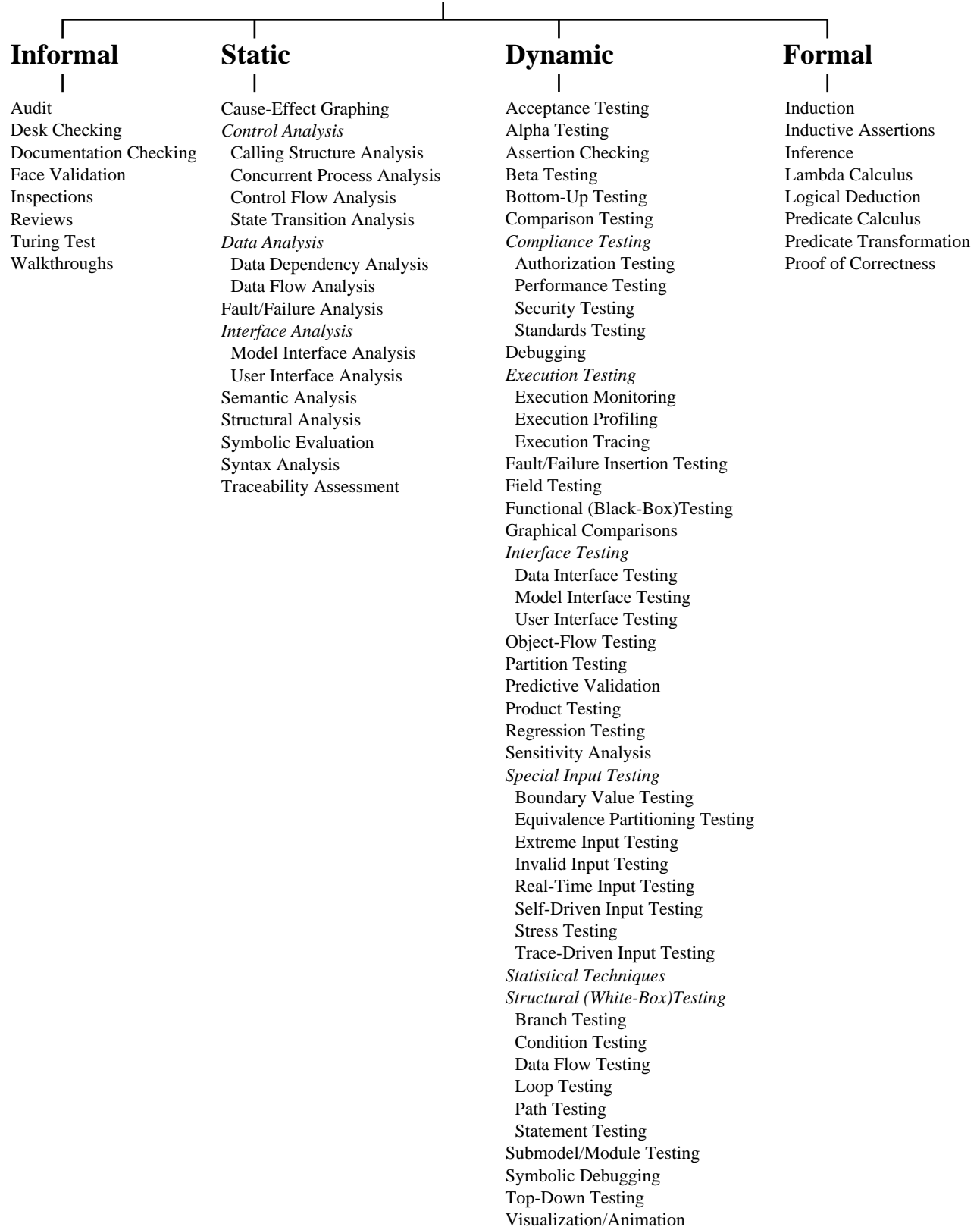
Figure 10.8. A Taxonomy of Verification, Validation and Testing Techniques.
