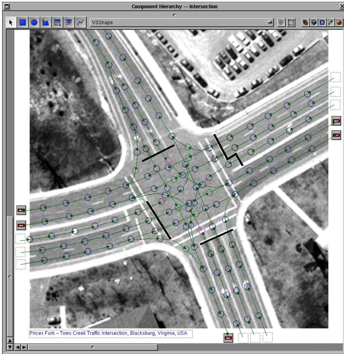
Figure 10.3. Model Specification in the Visual Simulation Environment.
