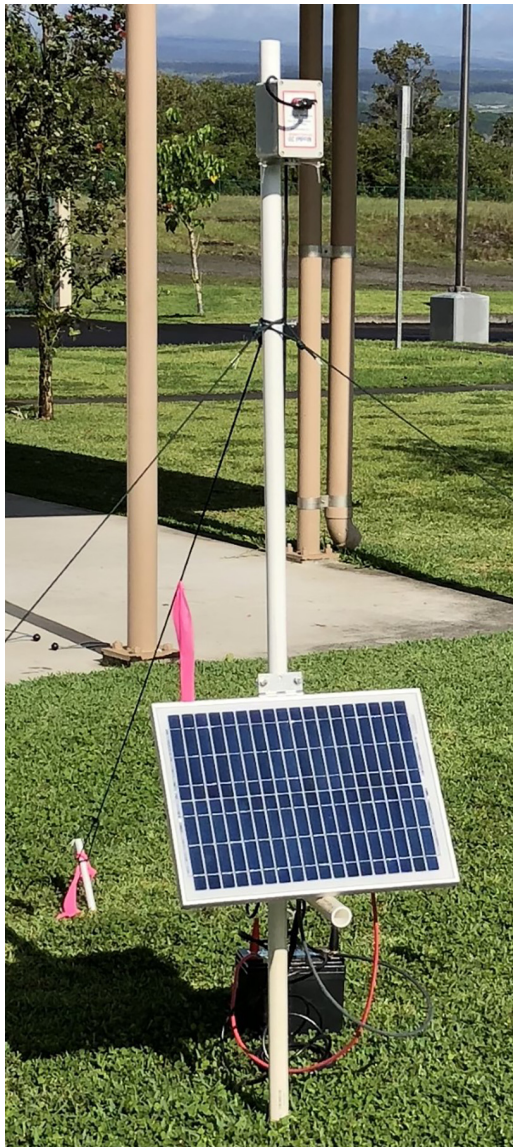
FIGURE 1 Rotorod sampler setup. Includes Model 20 Rotorod Sampler, rods pointing downward, mounted 1.5 m off the ground on PVC pipe, which also supports a 12V solar panel connected to a battery; stakes and three guywires support the setup.
