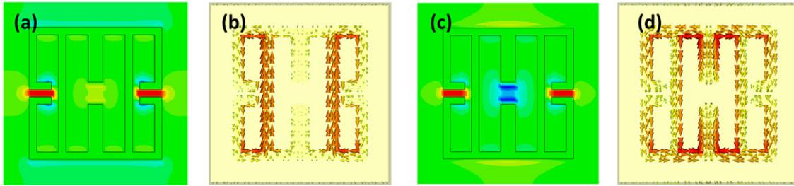
**Figure 3.** The electric field (a) and surface current distribution (b) at the lower frequency resonance of figure 2 (at 0.7 THz), and at the higher frequency resonance (electric field (c), and current (d)) at 1.38 THz.
