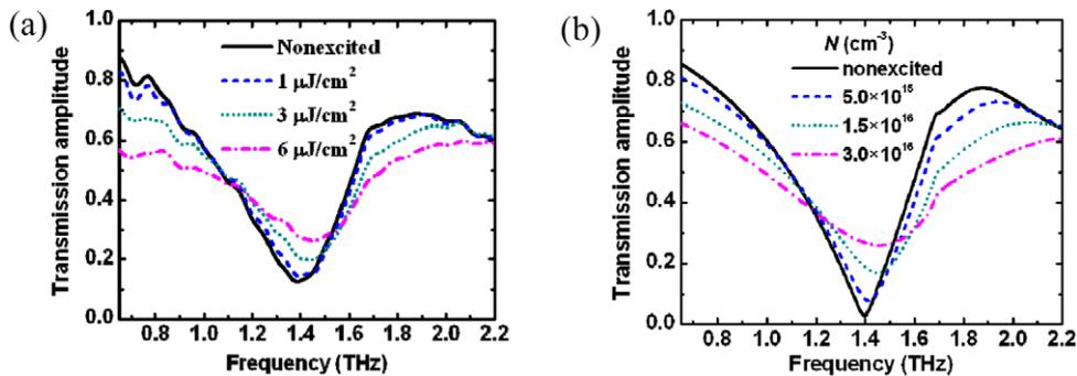
**Figure 9.** Experimental (a) and simulated (b) transmission amplitude spectra for different levels of photoexcitation of a system of SRRs (with geometrical features as described in figure 1(b)) on top of a GaAs substrate.
