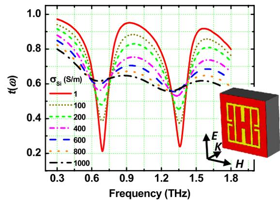
**Figure 2.** Simulated dual-band switching effect: transmission spectra as function of Si conductivity. The unit cell of the structure is shown in the inset; Si is marked with the red color.
