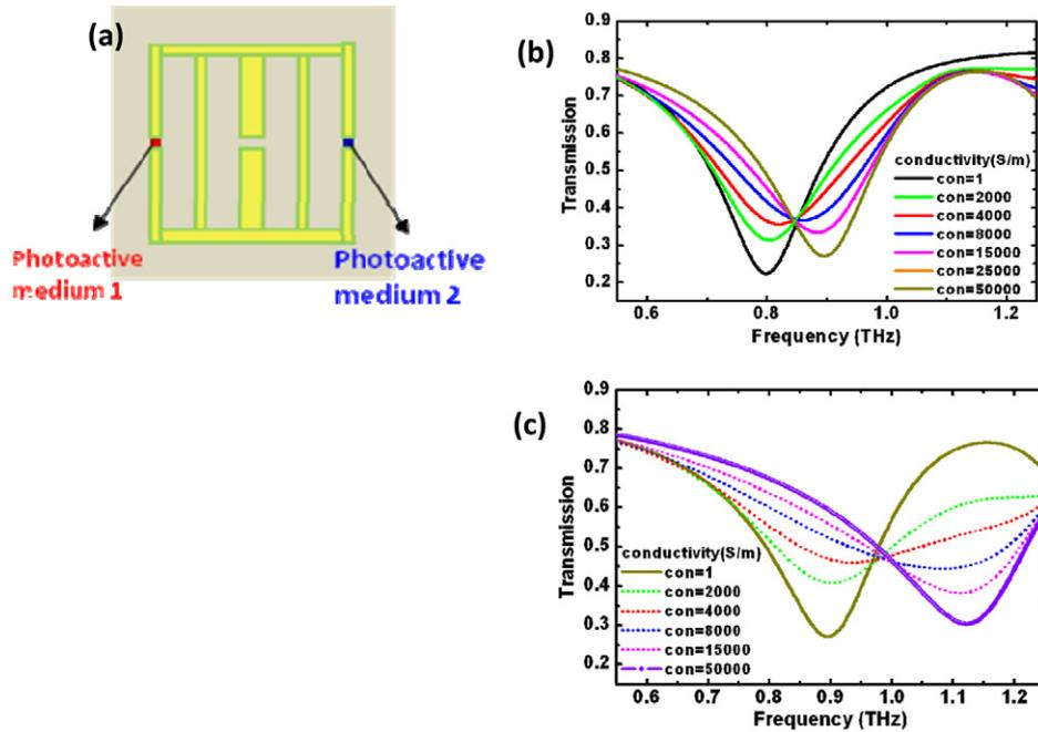
**Figure 8.** (a) The SRR design showing multi-mode switching. The geometrical parameters of the design are the same as in the one in figure 4. Numerical transmission spectra through a system of such SRRs for excitation of the photoconducting medium 1 (conductivity here refers to medium 1) (panel (b)), and medium 2, with medium 1 fully excited. Conductivity here refers to medium 2, while the conductivity of medium 1 has been taken as  $50\,000\text{ S m}^{-1}$  (panel (c)).
