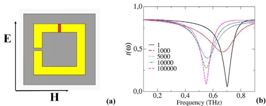
**Figure 7.** A two-gap single-ring SRR design showing red-shift tunability (a). The materials and dimensions are the same as the SRR of figure 1(b), with the inner ring missing. The gap size is  $2 \mu\text{m}$  for both gaps—one is filled with Si (red color). Panel (b) shows the numerical transmission spectra through a system of such SRRs for different values of the conductivity (mentioned in the legends—in  $\text{S m}^{-1}$ ) of the photoconducting Si.
