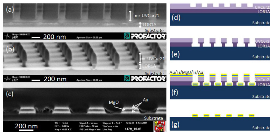
Figure 2. Cross-sectional SEM images (left) and schematic drawing of different process steps (right). (a), (d) Imprint into mr-UVCur21 on LOR1A layer. (b), (e) Imprint after etching and development to achieve recessed sidewalls. (f) Deposition of Au, Ti, MgO, Ti, Au. (c), (g) Final sample after lift-off.
