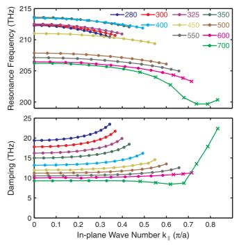
FIG. 9. (Color) As the experiment in Fig. 4, but derived from complete numerical calculations for actual infinite gold split-ring-resonator square arrays with lattice constants a, as indicated. Note the good qualitative agreement with the experiment in Fig. 4. The lateral geometry of the split-ring resonators is indicated in Fig. 1. The gold film thickness is 40 nm, and the glass substrate is accounted for.
