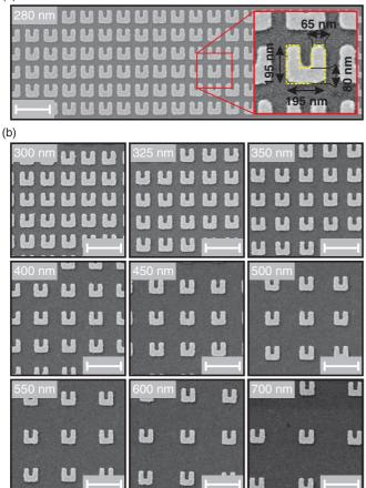
FIG. 1. (Color online) (a) Overview electron micrograph of the split-ring-resonator (SRR) square array with a = 280 nm lattice constant used in this paper. The total footprint of this array and all others is  $160 \ \mu m \times 160 \ \mu m$ . The SRR dimensions used for the numerical calculations are indicated in the inset. (b) Electron micrographs of all other SRR arrays in this work with lattice constants *a* as indicated. All arrays are shown on the same scale—the scale bar is 500 nm.
