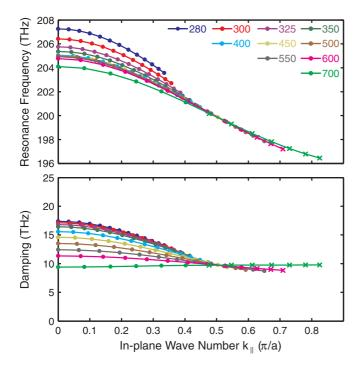
FIG. 7. (Color) Dispersion of center frequency and damping as derived from a chain of three electromagnetically interacting electric point dipoles in vacuum evenly separated by distance *a*, represented as the experimental data in Fig. 5. This treatment automatically accounts for retardation. The chain of three dipoles mimics short-range interaction only. Parameters are  $\Omega/(2\pi) = 200$  THz and  $\gamma/(2\pi) = 10$  THz. Note the disagreement with experiment in Fig. 4.
