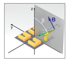
FIG. 2. (Color online) Illustration of the geometry used in our oblique-incidence optical transmittance experiments.
