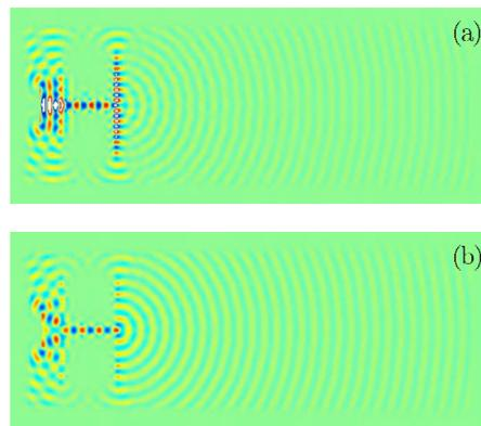
FIG. 5. (Color online) A 2D plot of the strength of the electric field of structure 3 at (a)  $f=11.97$  GHz and (b)  $f=11.33$  GHz.
