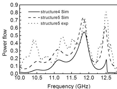
FIG. 7. Power flow versus frequency for structure 4 (simulation only) and structure 5 (simulation and experiment). Notice that structure 5 is similar to structure 4, except for the one grating missing in front at the end of the waveguide.
