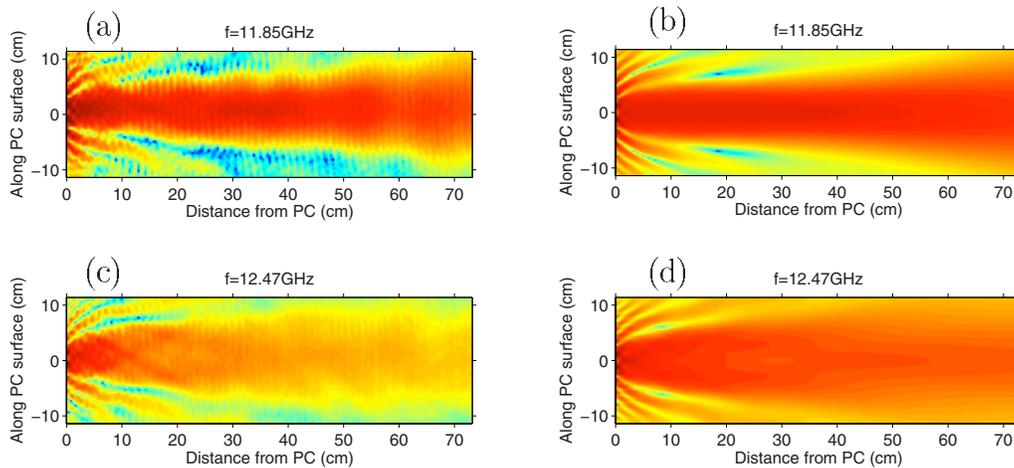
FIG. 11. (Color online) A 2D plot of the strength of the outgoing electric field for the case of structure 5. (a) and (b) are the experimental and the simulation results, respectively, at frequency  $f=11.85$  GHz. (c) and (d) are the experimental and the simulation results, respectively, at frequency  $f=12.47$  GHz.
