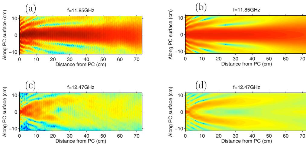
FIG. 10. (Color online) A 2D plot of the strength of the outgoing electric field for the case of structure 4. (a) and (b) are the experimental and the simulation results, respectively, at frequency  $f=11.85$  GHz. (c) and (d) are the experimental and the simulation results, respectively, at frequency  $f=12.47$  GHz.
