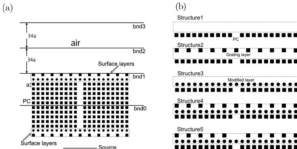
FIG. 1. (a) The structure’s details and definition of the different boundaries used.  $bnd0$ ,  $bnd1$ ,  $bnd2$ , and  $bnd3$  are the boundaries in the channel, at the end of the PC, in the middle of the air part and at the end of the air part respectively. (b) The shape of the surface layers in each of the five different structures.
