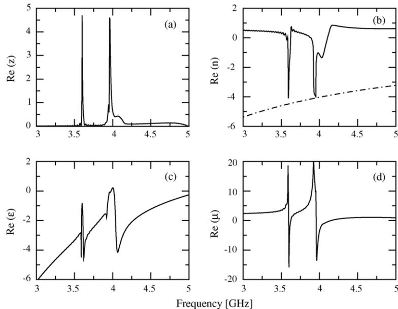
Fig. 4. The retrieved real part of the effective impedance,  $z$  (a), the refractive index,  $n$  (b), the electric permittivity,  $\epsilon$  (c), and the magnetic permeability,  $\mu$  (d), for the structure presented in Fig. 3, and for one unit cell in the propagation direction. The dot-dashed line shows the minimum value of the refractive index in the first Brillouin zone.
