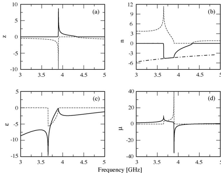
Fig. 2. The retrieved real (solid line) and imaginary (dashed line) parts of the effective impedance,  $z$  (a), the refractive index,  $n$  (b), the electric permittivity,  $\epsilon$  (c), and the magnetic permeability,  $\mu$  (d), for the structure presented in Fig. 1. The dot-dashed line shows the minimum value of the refractive index in the first Brillouin zone.
