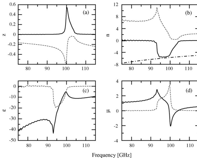
Fig. 6. The retrieved real (thick) and imaginary (thin) parts of the effective impedance,  $z$  (a), the refractive index,  $n$  (b), the electric permittivity,  $\epsilon$  (c), and the magnetic permeability,  $\mu$  (d), for the structure presented in Fig. 5. The dot-dashed line shows the minimum value of the refractive index in the first Brillouin zone.
