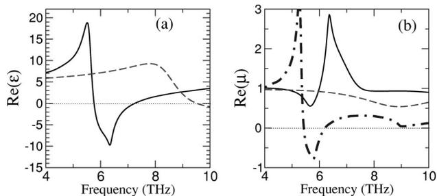
Fig. 4. (a) Real part of the effective permittivity of the SRR metamaterial shown in Fig. 1, for propagation direction and EM field polarization those of Fig. 1(d) (solid curve) and Fig. 1(c) (dashed curve). (b) Real part of the effective permeability of the SRR metamaterial for the orientations of Fig. 1(d) (solid curve), Fig. 1(c) (dashed curve), and Fig. 1(a) (dashed-dotted curve).
