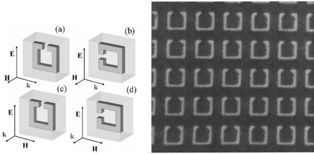
Fig. 1. Left, single unit cell of the SRR geometry studied, in all possible EM field propagation directions and polarizations [(a)–(d)]. Right, top view photograph of the SRR metamaterial fabricated by a microlithography process.
