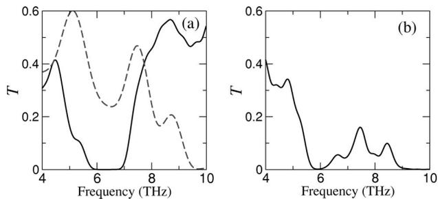
Fig. 3. (a) Calculated transmission versus frequency for the configurations shown in Figs. 1(c) (dashed curve) and 1(d) (solid curve). (b) Calculated transmission for the configuration in Fig. 1(a).
