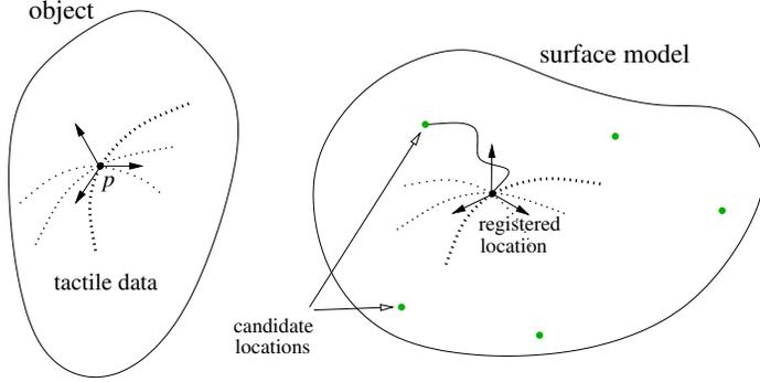
**Figure 1:** Registering three data curves on a surface. The grey (green) dots represent candidate locations of the curve intersection point  $p$  on the surface found in a table lookup. A search path leads from one of these locations to where the curves are “best” superposed onto the surface.
