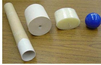
**Figure 7:** Objects used in the experiment: two regular cylinders with diameters 50.4mm and 94mm, respectively, an elliptic cylinder with semimajor axis 50.8mm and semiminor axis 31.75mm, and a sphere with radius 33mm.
