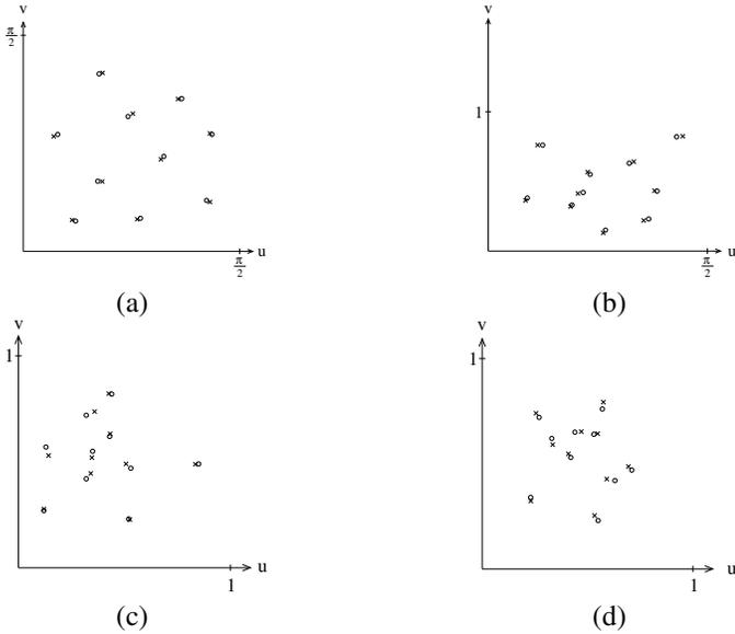
**Figure 6:** Instances of curve registration on the four shapes displayed in Figures 4 and 5: (a) an ellipsoid; (b) an elliptic paraboloid; (c) the monkey saddle; (d) the crossed trough. In each instance, the intersection point  $p$  of three data curves is represented by a circular dot and its estimated location  $p^*$  by the closest cross.
