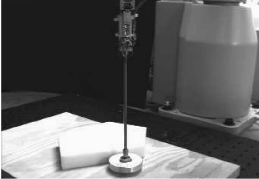
**Figure 15:** A force sensor for contact sensing. The sensor is composed of a horizontal disk with diameter 3cm and a cylindrical stainless steel beam erected vertically on the disk and attached to the gripper of an Adept robot at the top. Two pairs of  $350\Omega$  strain gauges are mounted on the upper end of the beam where they would be most sensitive to any force exerted on the disk. They measure the contact force along two orthogonal directions, respectively
