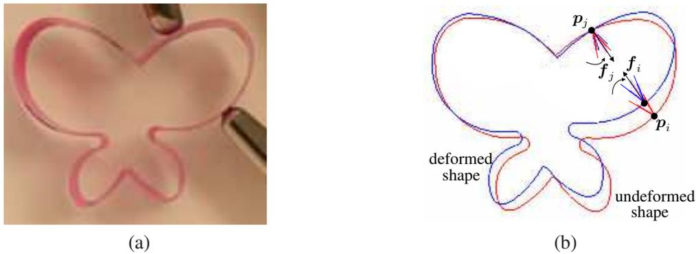
**Figure 15:** Rotations of two contact friction cones make the grasping forces more aligned in (a) experiment and (b) the corresponding simulation, where the arrows indicate the rotation directions.
