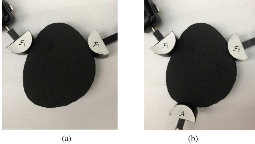
**Figure 12:** Experimental validation of the simulation result shown in Figure 10. (a) Grasp of a convex object corresponding to Figure 10(a). (b) Its resistance to an adversary finger  $\mathcal{A}$  corresponding to Figure 10(b). The translation  $\delta_2$  by  $\mathcal{F}_2$  in (a), and the translations  $\mathbf{d}_1$ ,  $\mathbf{d}_2$ , and  $\mathbf{a}$  by  $\mathcal{F}_1$ ,  $\mathcal{F}_2$  and  $\mathcal{A}$  in (b) are (straightened) from the trajectories in Figure 10(c).
