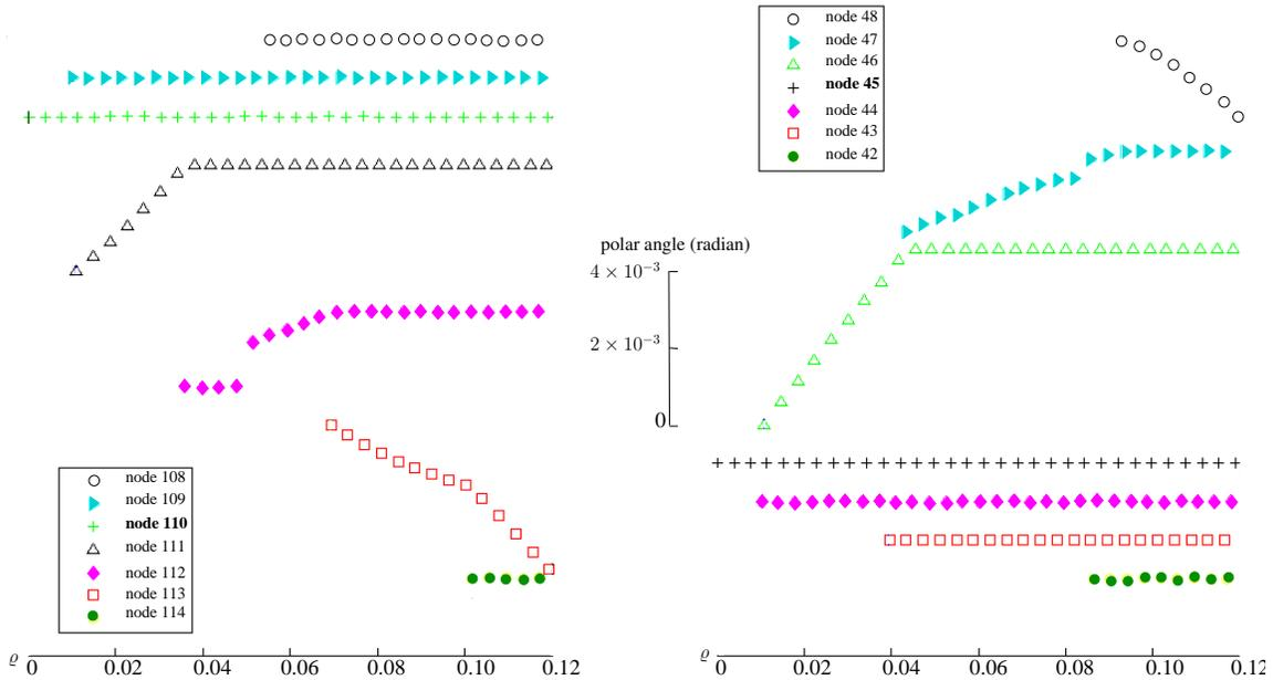
**Figure 6:** Trajectories (in polar angle) of the 14 contact nodes on the left and right fingertips in Table 1.
