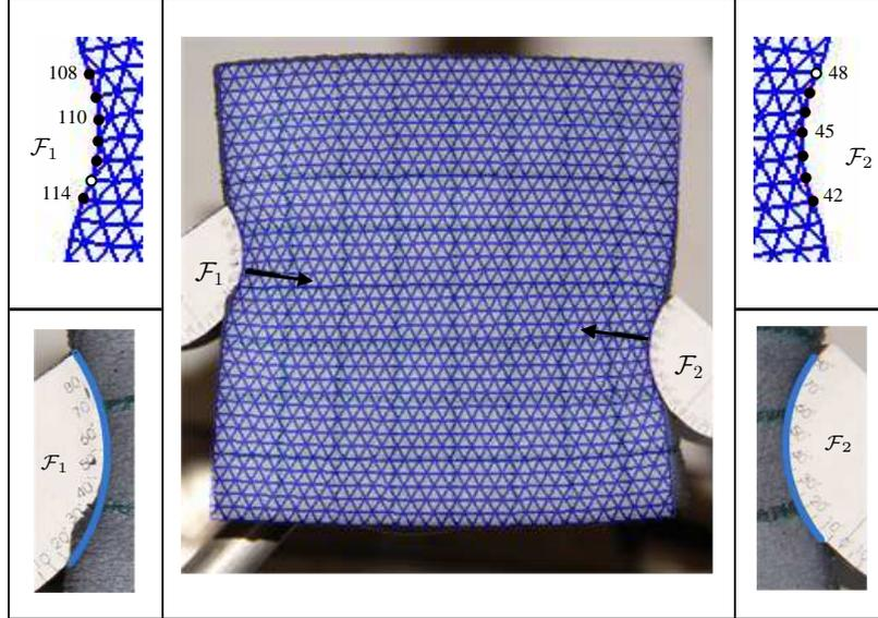
**Table 1:** Grasped foam rubber square with its deformed mesh superposed (center). The contact segments from simulation (row 1) each consist of six sticking nodes (solid dots) and one sliding node (hollow dot) numbered in the ranges 108–114 and 42–48, respectively. Nodes 110 and 45 were the initial contacts  $p_i$  and  $p_j$  with the two fingers. The contact segments in the experiment (row 2) are enlarged from the central image.
