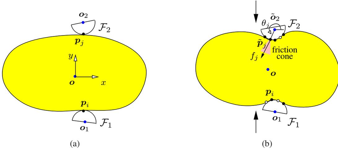
**Figure 5:** Object (a) before and (b) during a squeeze grasp. Solid dots represent the sticking contact nodes at the moment, while hollow dots represent the sliding contact nodes.
