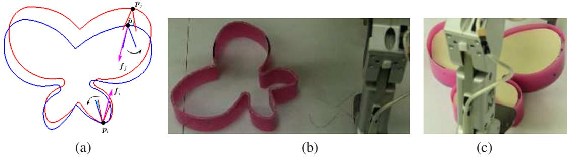
**Figure 14:** Grasp failure due to deformation at the relative squeeze depth of 15%. (a) Contact forces out of the friction cones. (b) Escape of the object. (c) Success at grasping a ‘rigid’ identical shape under the same finger placement.
