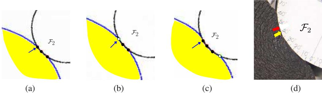
**Figure 7:** Transitions of a contact from (a) stick to (b) slip to (c) slick. Here (a) and (b) are the simulation results over the second object in Table 2 that correspond to its entries (2, 3) and (3, 3), respectively. In (c), the contact has stopped sliding, which is also observed in the experiment in (d).
