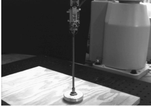
Figure 5: A force sensor for contact sensing. The sensor is composed of a horizontal disk and a cylindrical stainless steel beam erected vertically on the disk and attached to the gripper of an Adept robot at the top. Two pairs of strain gauges are mounted on the upper end of the beam where they would be most sensitive to any force exerted on the disk.
