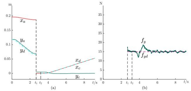
Fig. 8. Results for potato cutting. Trajectories of the (a) arm's free end  $\mathbf{a}$  and contact point  $\mathbf{c}$ , and (b) contact force between the knife and cutting board in the  $y$ -direction.
