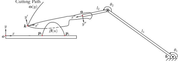
Fig. 2. Pressing by translating the knife downward.
