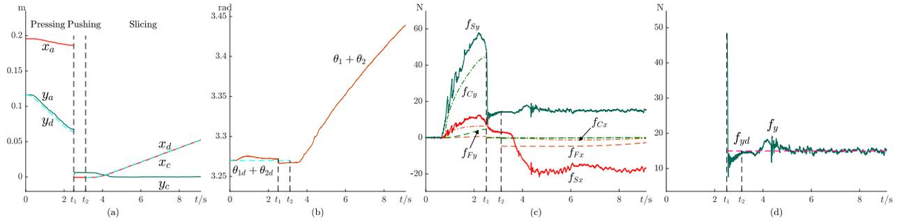
Fig. 7. Results from onion cutting. Trajectories of the (a) arm's free end  $\mathbf{a}$  and contact point  $\mathbf{c}$ , (b) sum of the two joint angles, (c) force  $\mathbf{f}_S = (f_{Sx}, f_{Sy})^T$  exerted on the knife as obtained from sensor readings, modeled fracture force  $\mathbf{f}_C = (f_{Cx}, f_{Cy})^T$ , and modeled frictional force  $\mathbf{f}_F = (f_{Fx}, f_{Fy})^T$ , and (d) contact force between the knife and cutting board in the  $y$ -direction.
