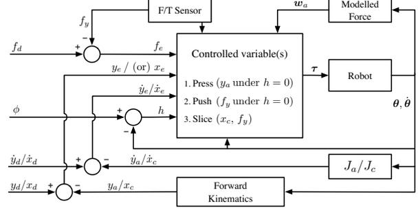
Fig. 3. Control diagram for three cutting phases.
