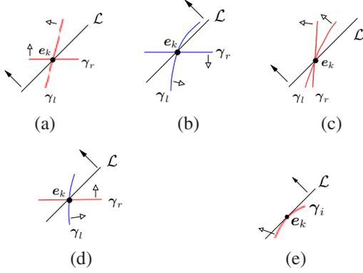
Fig. 7. Four types of intersection points: (a)  $(-, +)$ , (b)  $(+, -)$ , (c)  $(-, -)$ , and (d)  $(+, +)$ , and (e) an extremum point. A solid arrow shows the sweeping direction, while a hollow arrow marks the side where points define trajectories not in collision with the obstacle associated with the curve.
