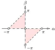
Fig. 3. C-space of trajectories  $\mathcal{T}(\alpha, \beta)$  that take the sphere from the origin to a point on the positive  $x$ -axis. The space consists of two open triangular regions bounded by the two axes and the lines  $\alpha - \beta = \pi$  and  $\beta - \alpha = \pi$ .
