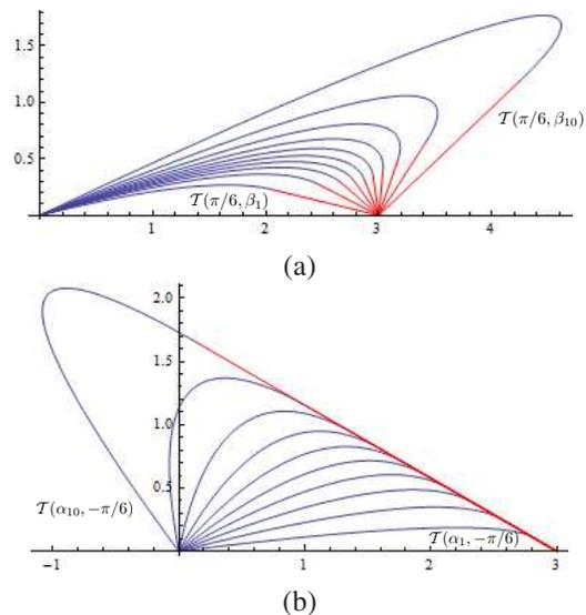
Fig. 4. Two groups of 10 trajectories each from the origin to  $(3, 0)$  with (a) the same sliding angle  $\alpha = \pi/6$  but different rolling angles  $\beta_i = -\frac{i}{11}(\pi - \alpha)$ ,  $1 \leq i \leq 10$ ; and (b) the same rolling angle  $\beta = -\pi/6$  but different sliding angles  $\alpha_i = \frac{i}{11}(\beta + \pi)$ ,  $1 \leq i \leq 10$ .
