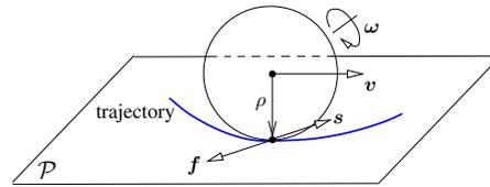
Fig. 1. Contact velocity  $s$  of a sphere and contact frictional force  $f$ .
