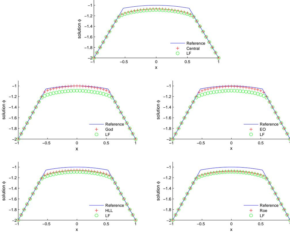
Figure 7: Resolution of discontinuities for 1st order, example 4.3 for  $T = 1$ , 40 cells, on the whole domain  $-1 \leq x \leq 1$ .
