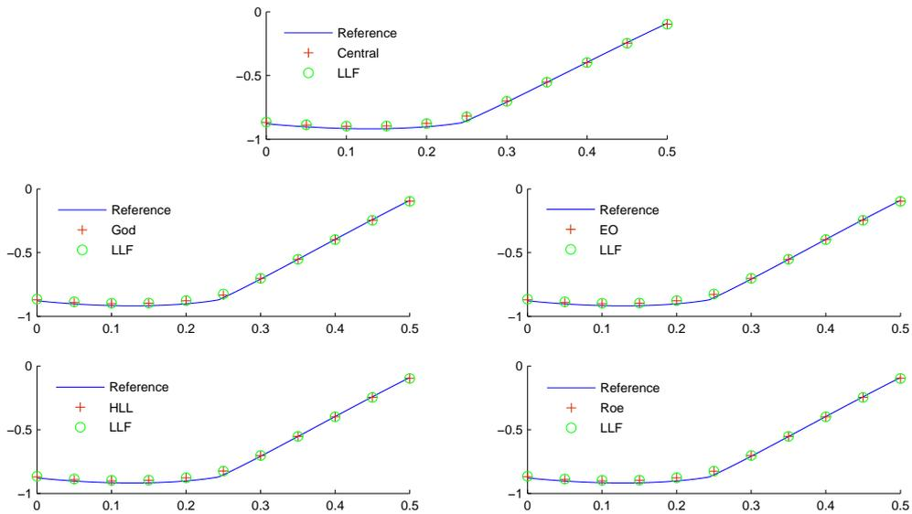
Figure 4: Resolution of discontinuities for 1st order, example 4.2 for  $T = \frac{1.5}{\pi^2}$ , 40 cells, zoomed at the region  $0 \leq x \leq 0.5$  which contains the discontinuous derivative in the solution.
