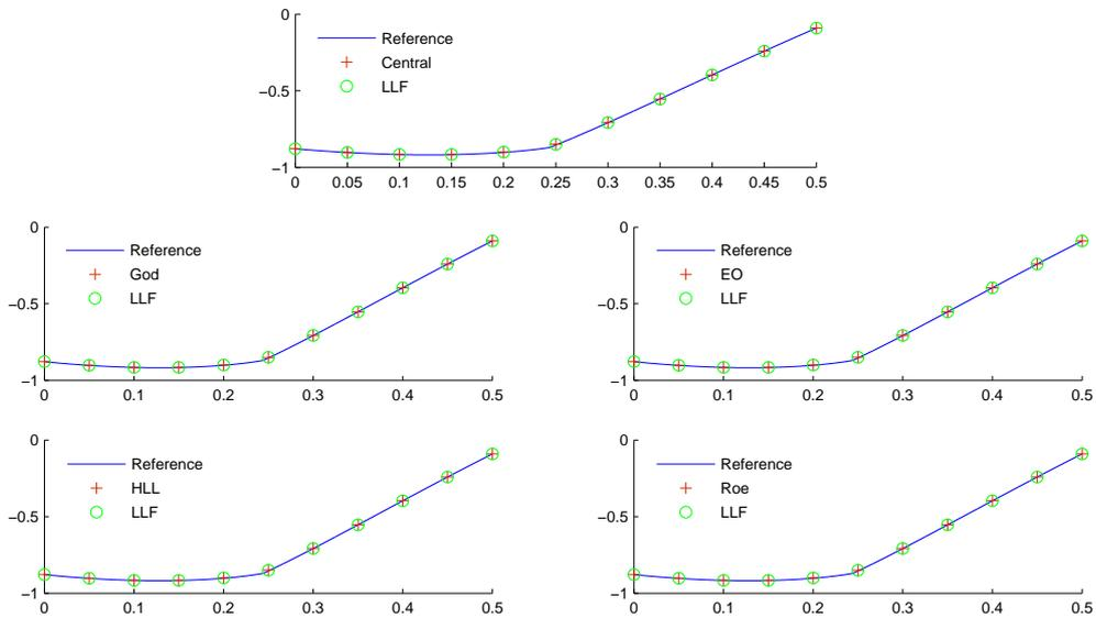
Figure 6: Resolution of discontinuities for 3rd order, example 4.2 for  $T = \frac{1.5}{\pi^2}$ , 40 cells, zoomed at the region  $0 \leq x \leq 0.5$  which contains the discontinuous derivative in the solution.
