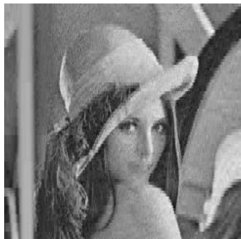
Figure: generalized Walsh Lena, 88% components removed, 243 by 243
