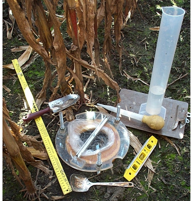
Figure 2: At left, the scoop method of soil bulk density measurement. At right, the USDA method of soil bulk density measurement.
