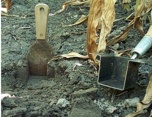
Figure 2: At left, the scoop method of soil bulk density measurement. At right, the USDA method of soil bulk density measurement.
