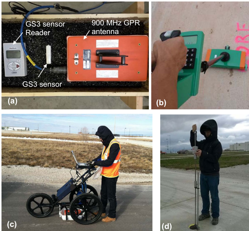
Figure 1. (a) Test setup using GS3 sensor and GPR antenna in laboratory box study; (b) MIT gauge; (c) GPR setup with a scanning survey wheel setup in situ ; and (d) DCP testing of the foundation layer through a pavement core.
